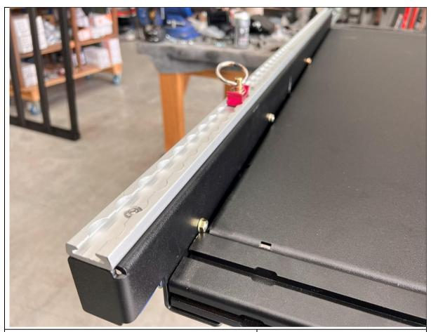
27. Finish putting all 4 screws per side securing the tray to the slides.
