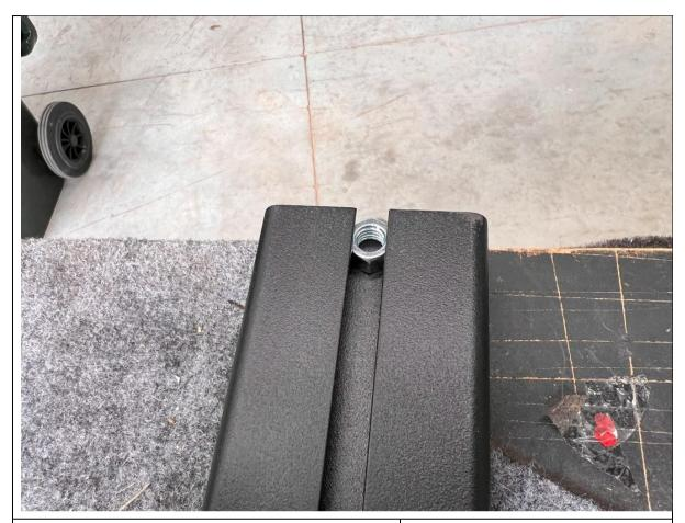
9. Fit 2 x M8 nuts per side into 1275mm extrusion.
